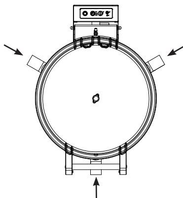
b) Water drainage outlet. Minimum diameter 35 mm (1 3/8 in). When connecting the drainage avoid bends and slopes.
