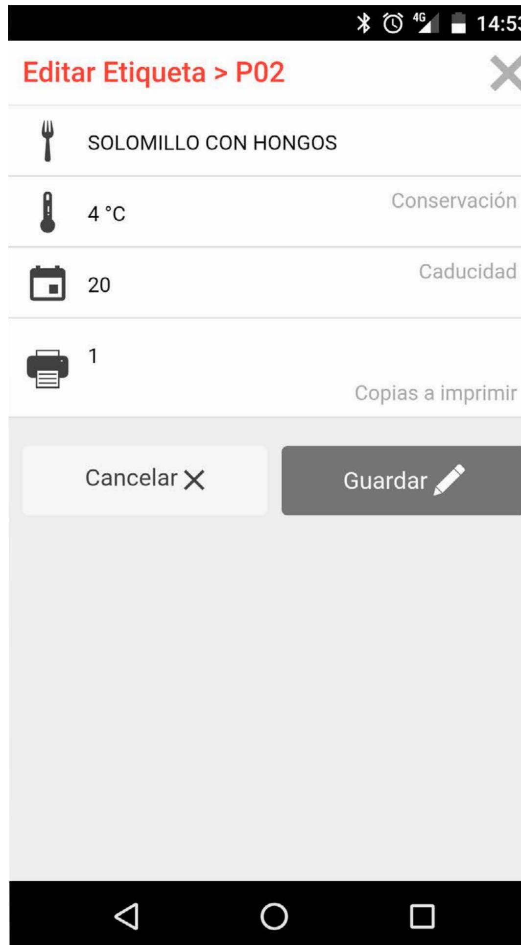
The introduction of texts for labelling is done via the SammicVAC app and is transmitted to the vacuum packer. The name of the recipe, the expiry dates, storage temperature and the values of the packaging programme are introduced. The labels are printed automatically and in the requested quantity, at the end of the cycle.
