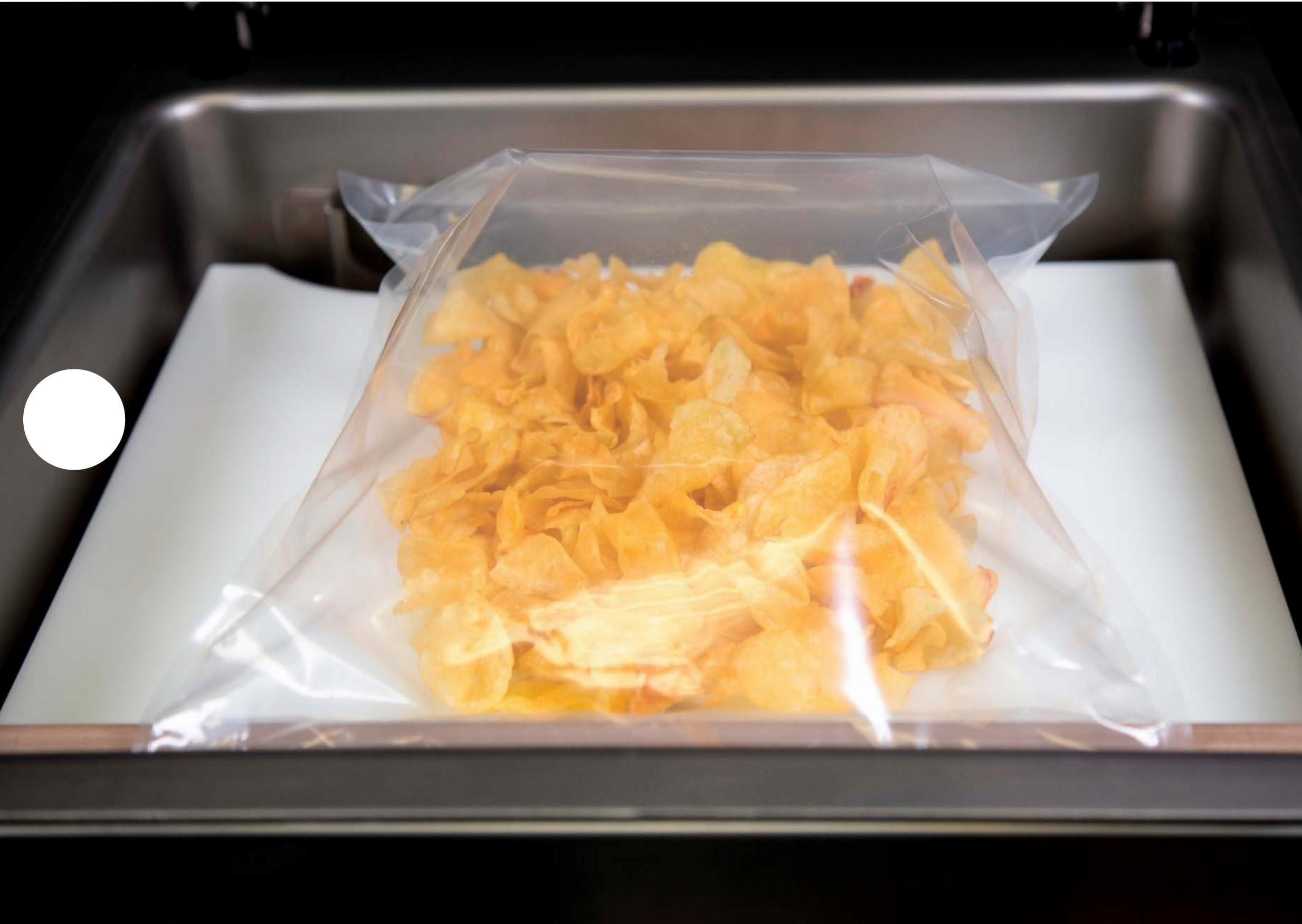
The installation of the inert gas injection system is optional on all models. This function allows you to package in a protective atmosphere. Depending on the gas employed and the product to be packaged, it obtains enhanced conservation of the product, improvement in its appearance and avoids damage in the case of fragile products.
