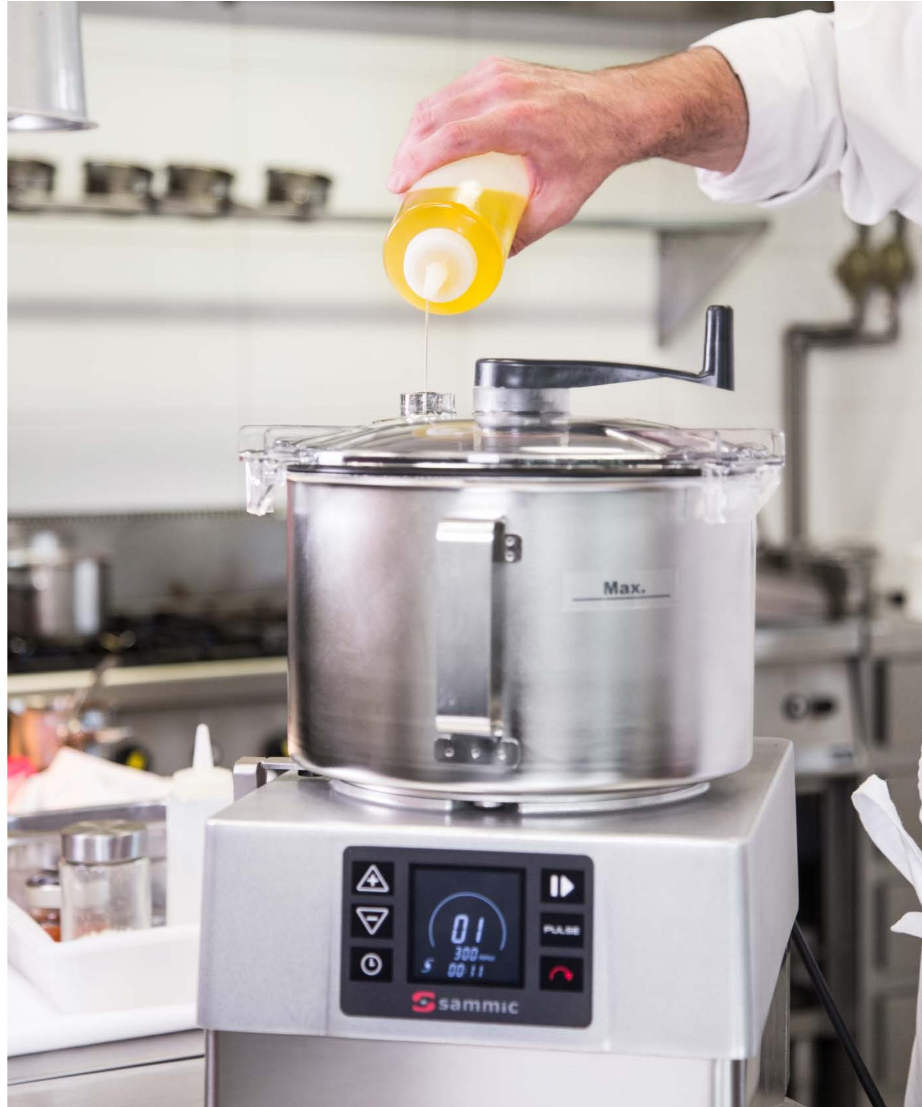
The cutter bowl's cover has an opening through which ingredients can be added during the cycle. The opening has a cover that can be closed when it is not being used, thereby avoiding splashing.
