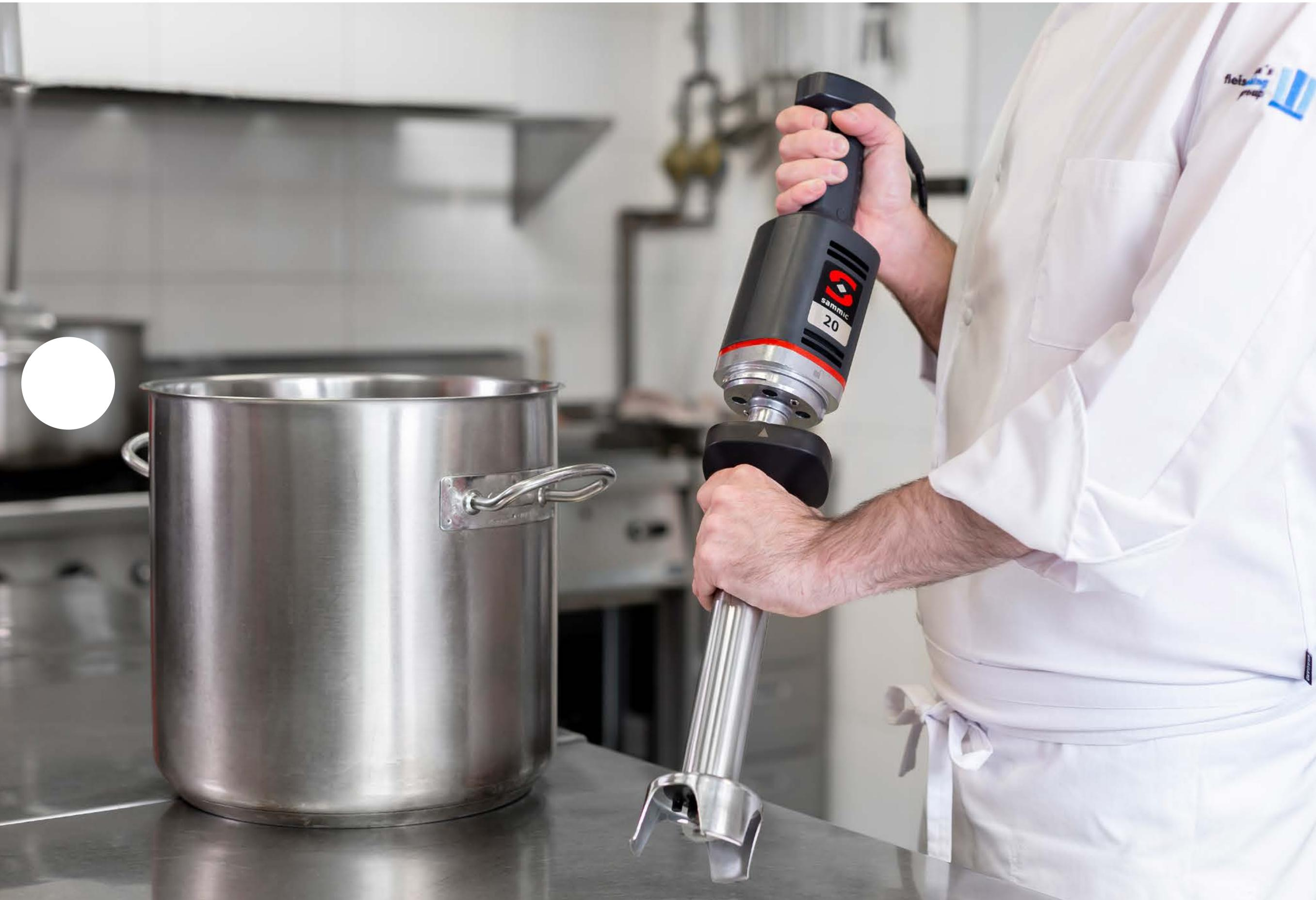
The arm is **detachable** with quick fastening due to the safety restraint system and the “click” which indicates the locked position.
