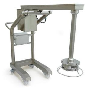
Turbo-blender designed to work in up to 800 I / 130 gal
